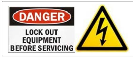
Never assume that any circuit is safe to work on until you are sure that it is de-energized. Make sure that it cannot be accidentally re-energized after you begin working on it. Follow your facility or OSHA Lockout/Tagout (LOTO) procedures ANYTIME maintenance or service is being performed on any electrical box or component. Affix a lock and warning tag on disconnects, breakers, and/or pulled fuses to alert others!
