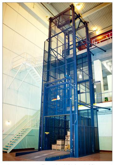
and support structure. The carriage is fabricated of 6" structural members with a steel deck plate. Additional deck surfaces are available. An electric motor/reducer assembly, which is mounted to the guide columns, lifts and lowers the carriage.
