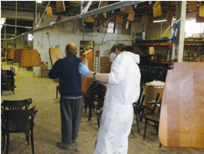
Sanding is done while parts are hanging.
