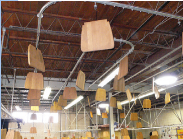
Conveyor loops at ceiling elevation and takes advantage of the warmer air space to speed up dry time.
