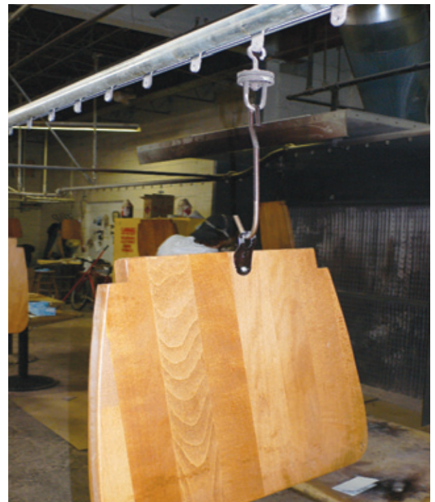
A convenient clip is attached to the wood part to allow handling.
