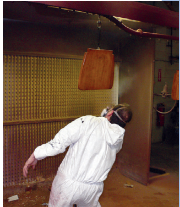
Part rotators and “in-booth” elevation changes allow operators convenient access to all sides of parts.
