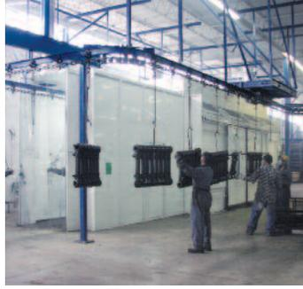
Wet spraying of heavy truck suspension components on the **PAC-BEAM™** trolley conveyor.
