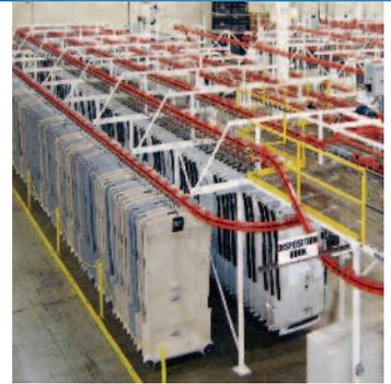
Automotive parts in a **PACLIN** Power and Free live storage system allows for unexpected production stoppages at supplier without impacting on final auto assembly plant.
