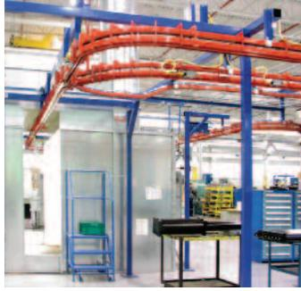
Wet spray painting of pneumatic cylinders using the **PACLIN** Power and Free conveyor.
