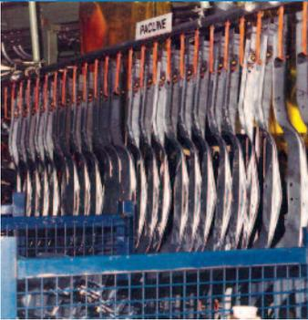
Manual, over/under parts buffer loop for automotive frames. Parts transferred from work station to work station using the **PAC-LINE™** conveyor system.
