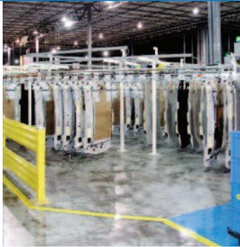
Automotive components stored in the **PAC-LINE™** automated storage and retrieval system facilitates batch building, retrieve to broadcast.
