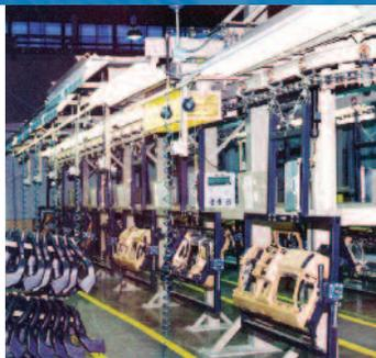
Automotive instrument panels transported through assembly process on the **PAC-BEAM™** overhead conveyor system with ergonomic carriers that tilt.
