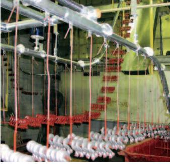
Dip paint finishing of lifting hooks in confined area with steep elevation changes using the **PAC-LINE™** enclosed track conveyor.
