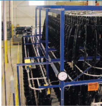
Unfinished automotive components accumulating on a multi-level **PAC-LINE™** enclosed track conveyor.
