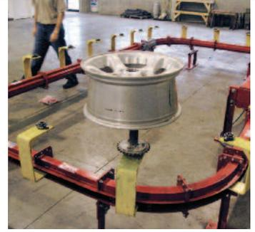
Finishing of automotive rims on rotating spindles using "slot sideways" enclosed track **PAC-MAX™** conveyor.
