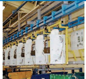
Assembly of high efficiency furnaces on the **PACLIN** Power and Free conveyor.
