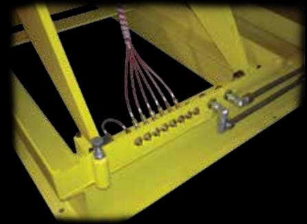
Central lube point
