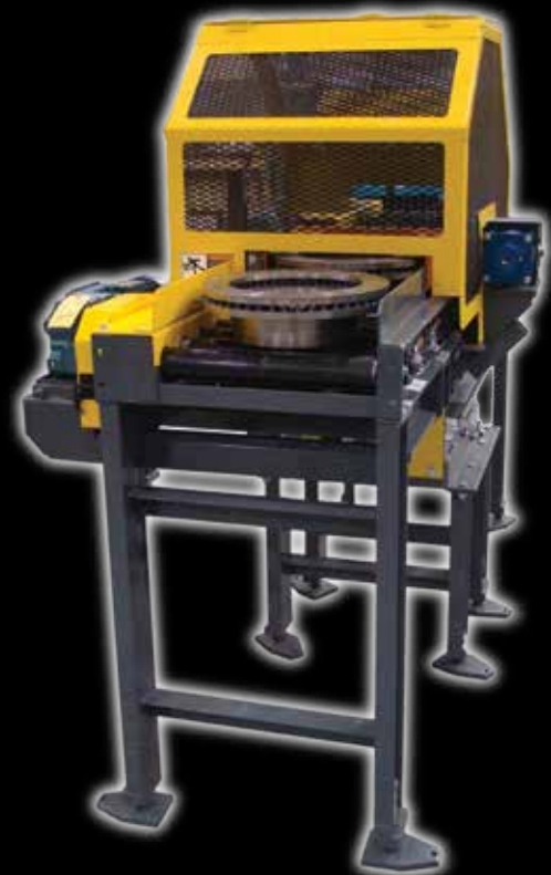
■ Infeed and outfeed chain driven live roller conveyor
