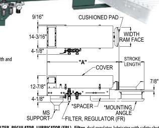
FILTER, REGULATOR, LUBRICATOR (FRL)—Filter, dual regulator, lubricator with safety shut-off valve, % in. NPT inlet port.
