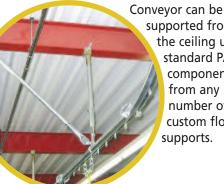
supported from the ceiling using standard PACLINE components or from any number of custom floor supports.
