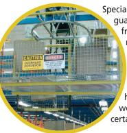
Special protective guarding made from nylon mesh, steel mesh or sheet metal may be added to a system to help ensure worker safety in certain situations.
