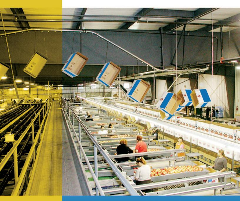
Overhead Conveyors for Produce Packing Operations
