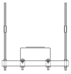
NOTE: Coupling Nut for Over 8 ft. Long Rods
